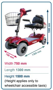
Size: fits in an allocated space of 1300mm by 800mm.
